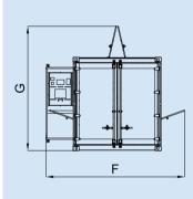
Installation dimension diagram (bottom view of base)
